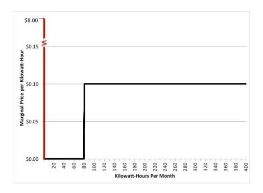
Illustration of Rate Structure with Minimum Bill (Min Bill \$8, p=\$0.10/kWh)
